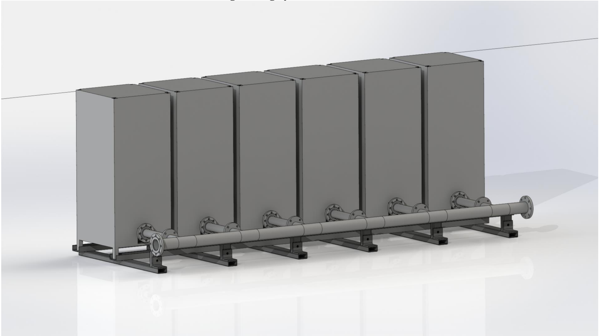
Figure A4.9 Installation of a module with a lower output for a centralized automatic gas-powder fire extinguishing system.
